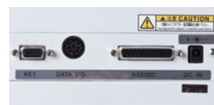
Data transfer port of AUW/AUX/AUY Series
