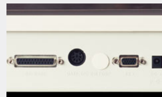
Data transfer port of BW-K/BX-K Series
